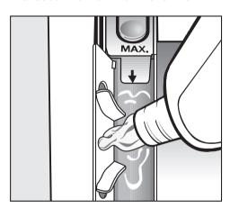
It will be automatically dispensed in the last rinse. At the end of the programme a small amount of water remains in the fabric conditioner compartment &.
